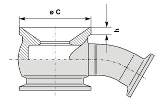
5.2 dimensions in mm for the tank bore
